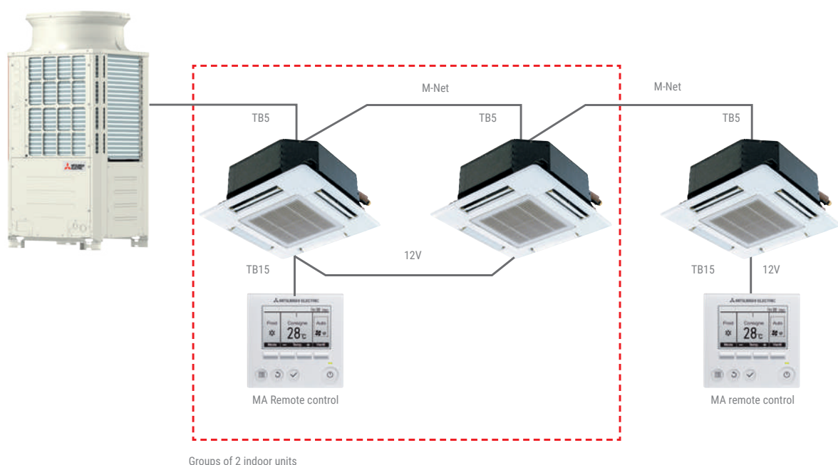
EXAMPLE OF WIRED CONNECTION (MA controller)
