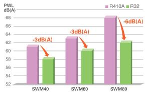
\*Compared SUZ-SWM40/60/80VA with SUHZ-SW45VA/PUHZ-SW50VKA/PUHZ-SW75VHA
