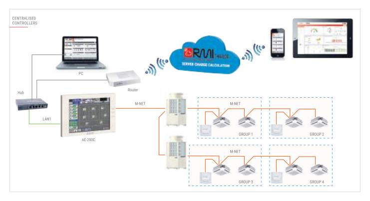
The RMI CHARGE cloud based system is capable of acquiring, calculating and apportioning consumption of the following energy utilities:
