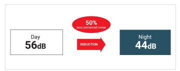
\* In Silent Mode, the thermal and/or cooling capacity of the outdoor unit is limited.
