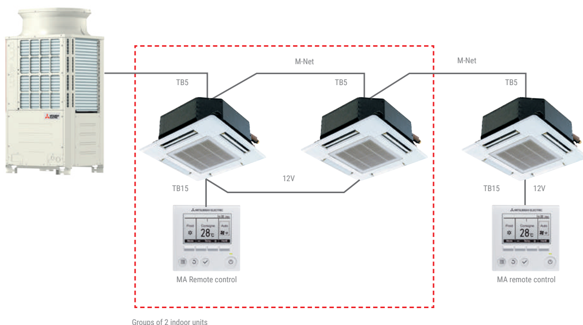
EXAMPLE OF WIRED CONNECTION (MA controller)
