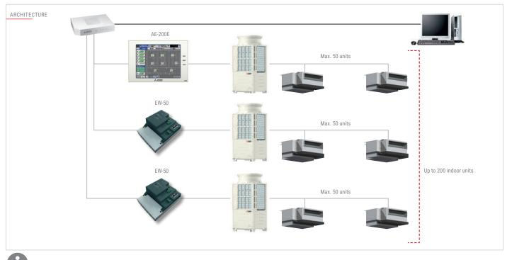
If the AE-200 is not used, up to four EW-50 units may be connected.
