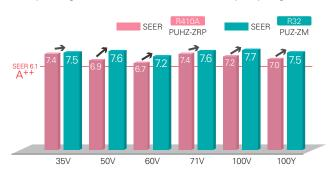
Introduction of new R32 refrigerant reduces energy consumption and realises energy savings.
