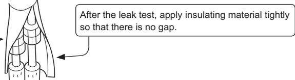
When the piping is to be attached to a wall containing metals (tin plated) or metal netting, use a chemically treated wooden piece 20 mm or thicker between the wall and the piping or wrap 7 to 8 turns of insulation vinyl tape around the piping. To use existing piping, perform COOL operation for 30 minutes and pump down before removing the old air conditioner. Remake flare according to the dimension for new refrigerant.
