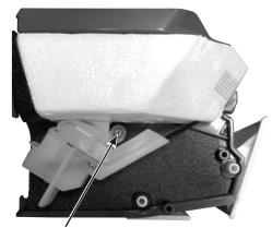
Screw of the vertical vane motor unit
