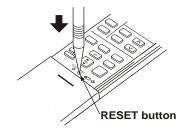
NOTE: 1. If RESET button is not pressed, the remote controller may not operate correctly.
