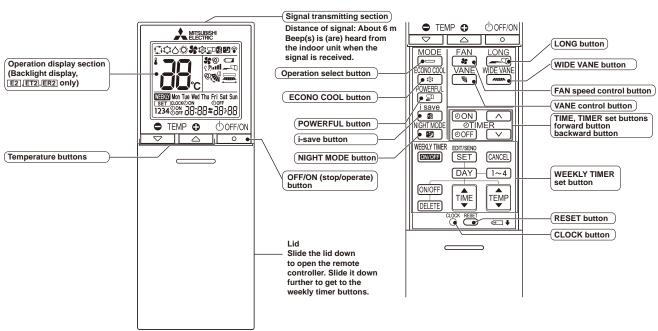
**NOTE**: Last setting will be stored after the unit is turned OFF with the remote controller. Indoor unit receives the signal of the remote controller with beeps.
