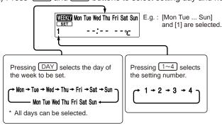
(3) Press ON/OFF , and ाक्षी buttons to set ON/OFF, time, and temperature.
