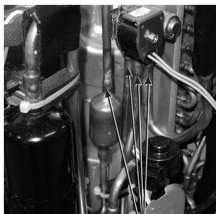
Brazed parts of 4-way valve
