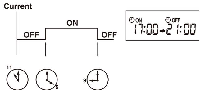
**NOTE:** If the main power is turned OFF or a power failure occurs while ON/OFF timer is active, the timer setting is cancelled. As these models are equipped with an auto restart function, the air conditioner starts operating with timer cancelled when power is restored.
