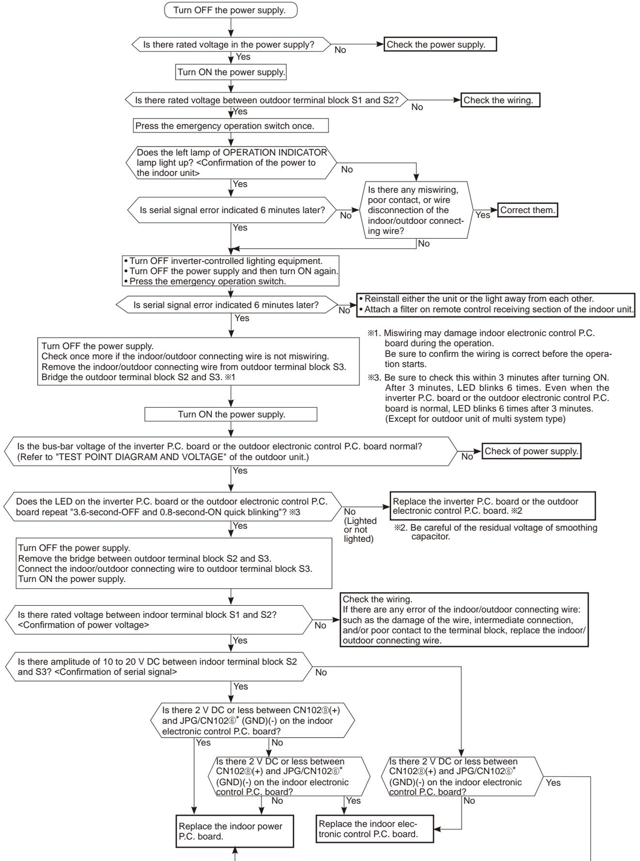
※1. Miswiring may damage indoor electronic control P.C. board during the operation. Be sure to confirm the wiring is correct before the operation starts.
