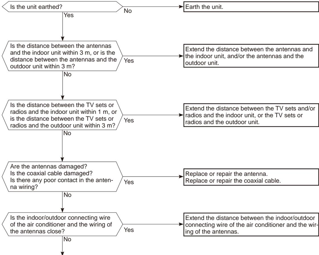
Even if all of the above conditions are fulfilled, the electromagnetic noise may enter, depending on the electric field strength or the installation condition (combination of specific conditions such as antennas or wiring).
