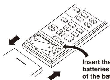
Insert the negative pole of the batteries first. Check if the polarity of the batteries is correct.
