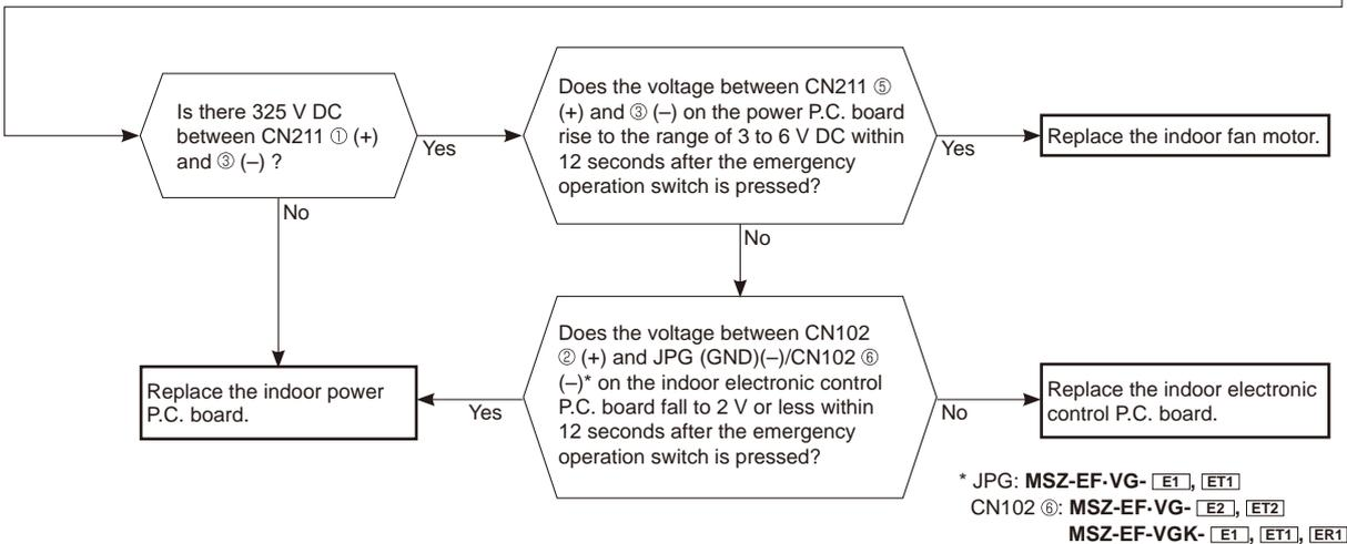
The indoor fan motor error has occurred, and the indoor fan repeats "12-second ON and 30-second OFF" 3 times, and then stops.
