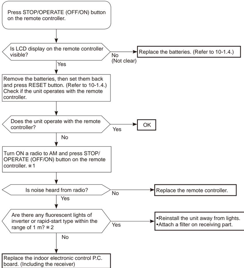
※ 1 Look at the image of the signal transmitting section of the remote controller through the monitor of a digital camera or a camera phone. It is normal if the LED of the signal transmitting section lights up when the STOP/OPERATE (OFF/ON) button on the remote controller is pressed. However, it may be difficult to see the illuminated LED of the signal transmitting section with a smartphone camera.
