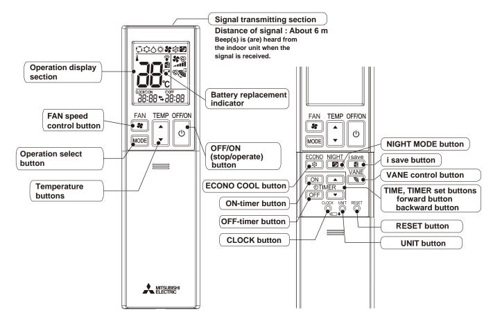
**NOTE**: Last setting will be stored after the unit is turned OFF with the remote controller. Indoor unit receives the signal of the remote controller with beeps.
