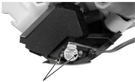
Screws of the vane motor
