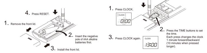
NOTE: 1. If RESET button is not pressed, the remote controller may not operate correctly.
