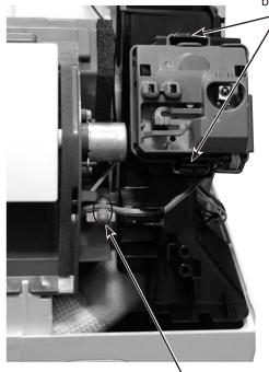
Fixing band of the vane motor wire
