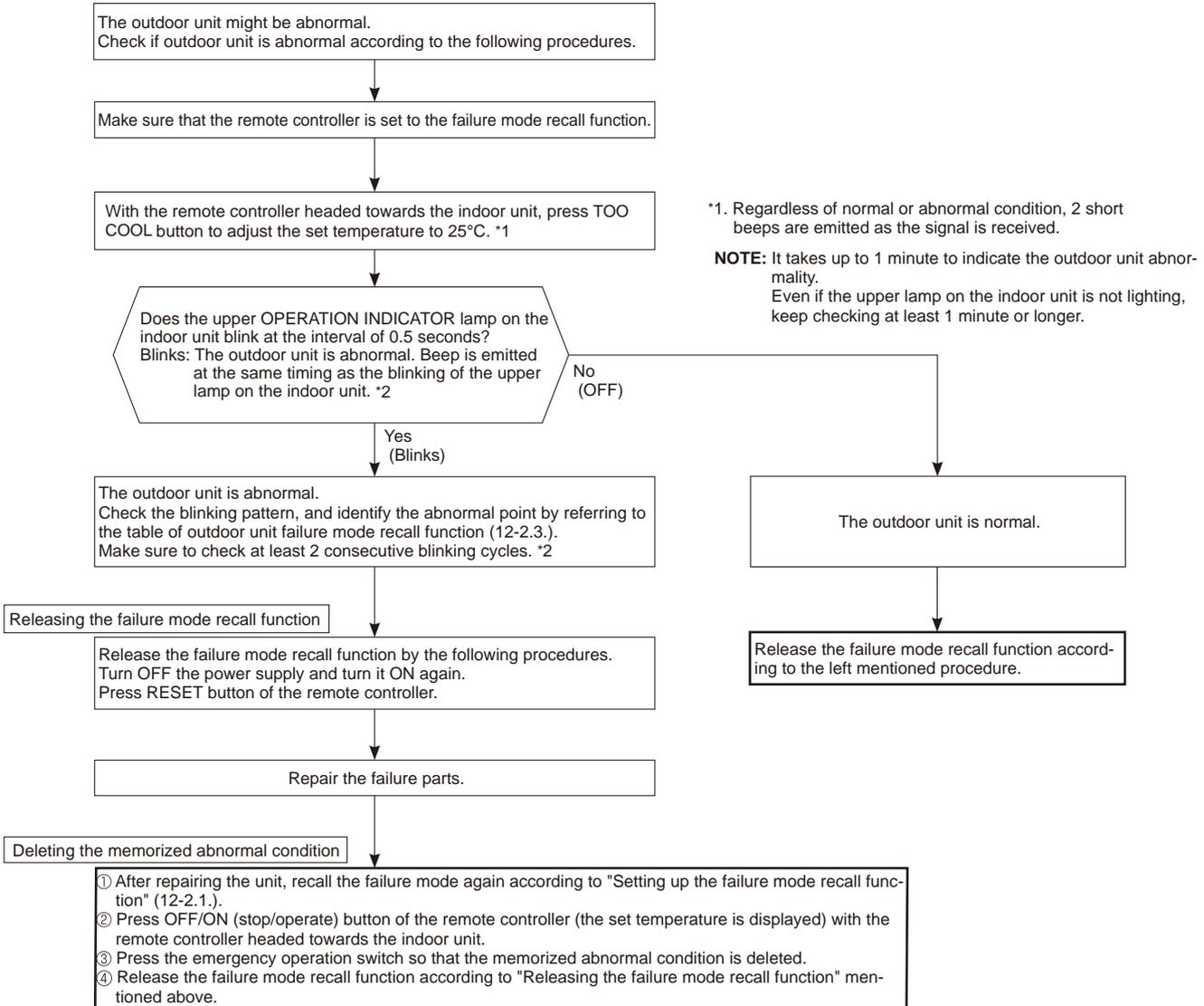
**NOTE:** 1. Make sure to release the failure mode recall function after it is set up, otherwise the unit cannot operate properly.
