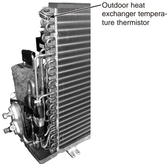
Outdoor heat exchanger temperature thermistor
